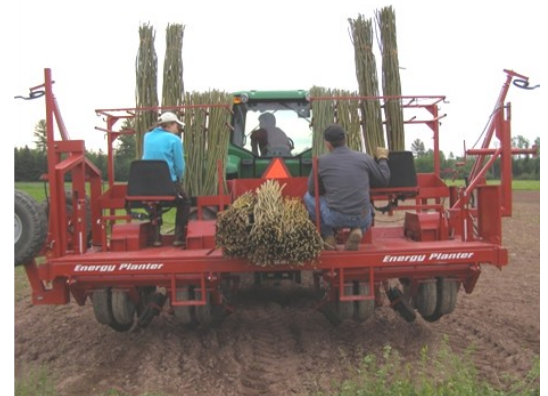
The Energy Planter was used to mechanically plant 8" cuttings. With good soil conditions, the planter works efficiently and quickly.
